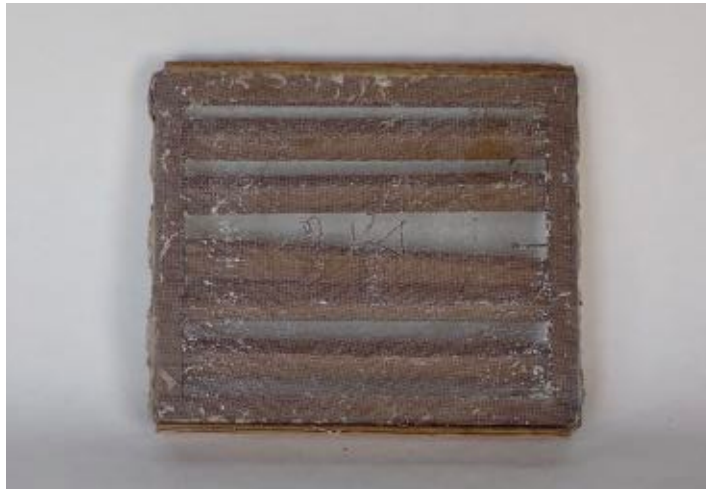
RPF2 mould, aluminum window screen
